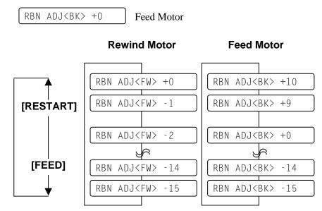
**[FEED]** key: Pressing the **[FEED]** key one time causes a -1 step change, up to -15 steps.
